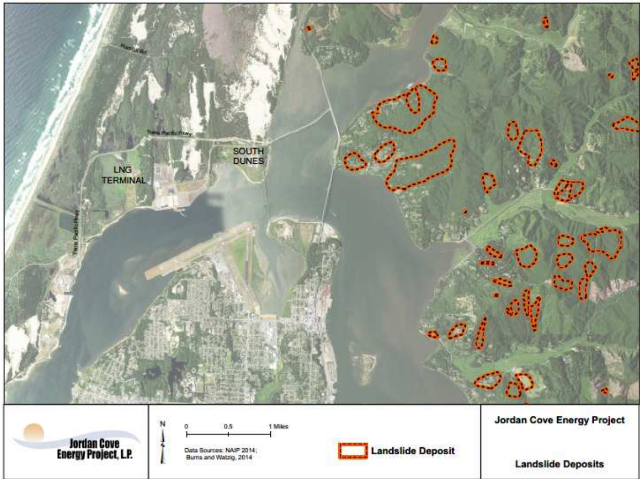
Figure 6.4-2: Mapped Landslide Deposits
